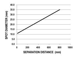
Figure 6. Spot Diameter Diagram
