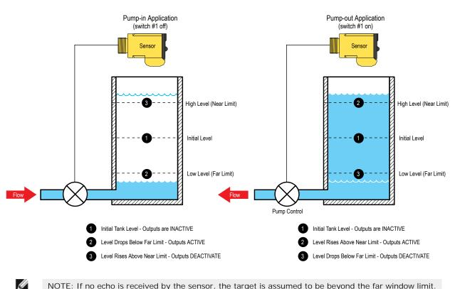
NOTE: If no echo is received by the sensor, the target is assumed to be beyond the far window limit.
