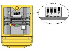
Figure 2. Q45U Programming Switches
