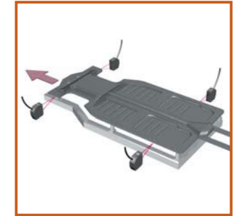
Measuring Car Body Widths (ZS-HLDS10)
