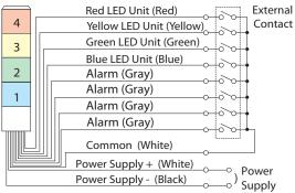
$\Theta$  KJ-110/112/120 are voltage-contact type, therefore have no alarm signal wires.
