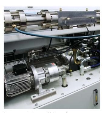
Pressure monitoring on a high-speed pump
